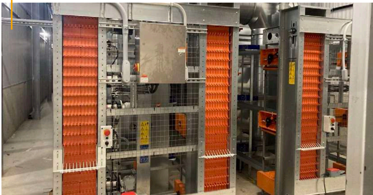
Egg gathering with elevators for the group cages.
