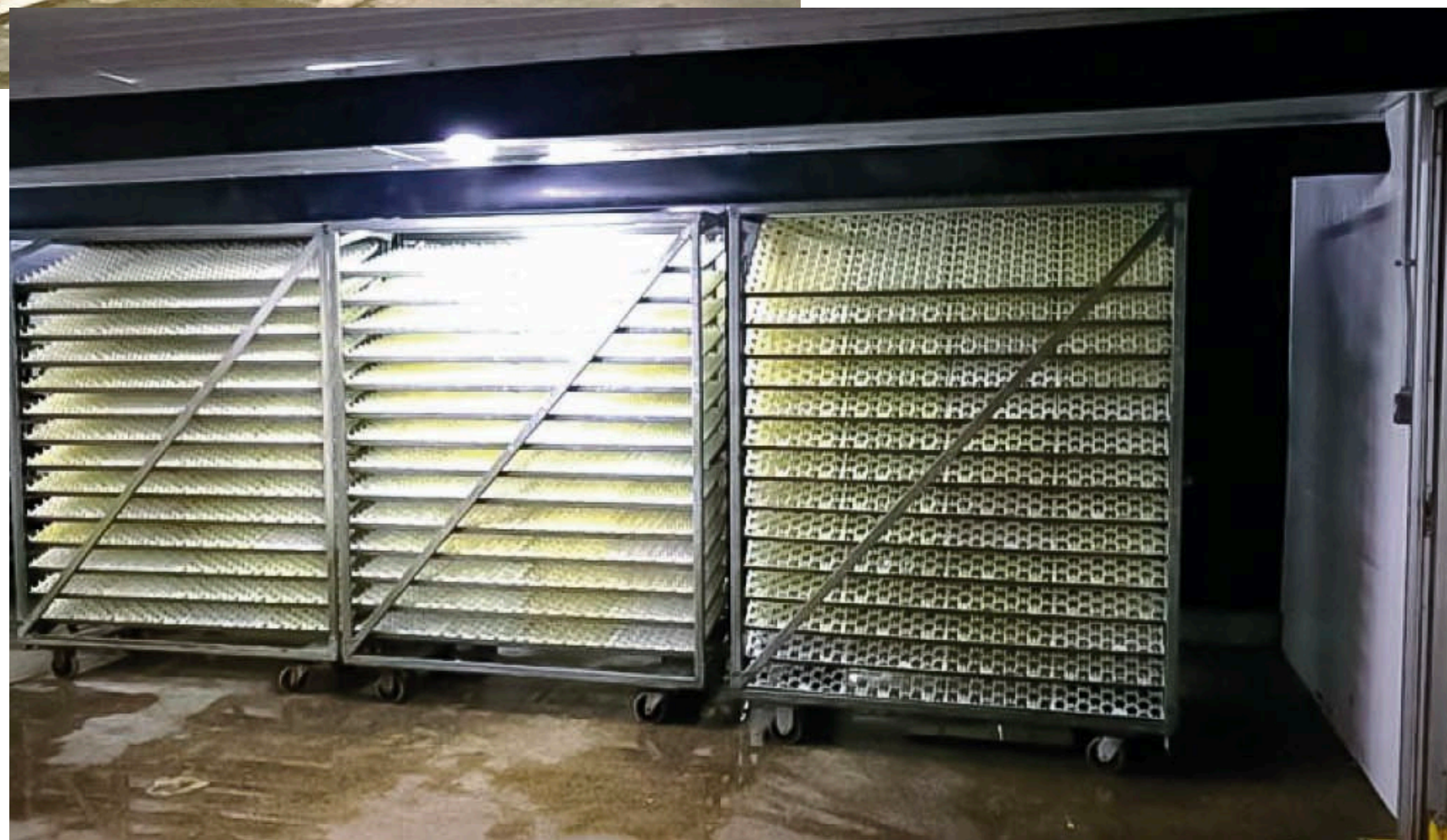
▼ Image 2. Actual pre-warming room for 300.000 eggs at once, showing the deflectors and trolley disposal.
