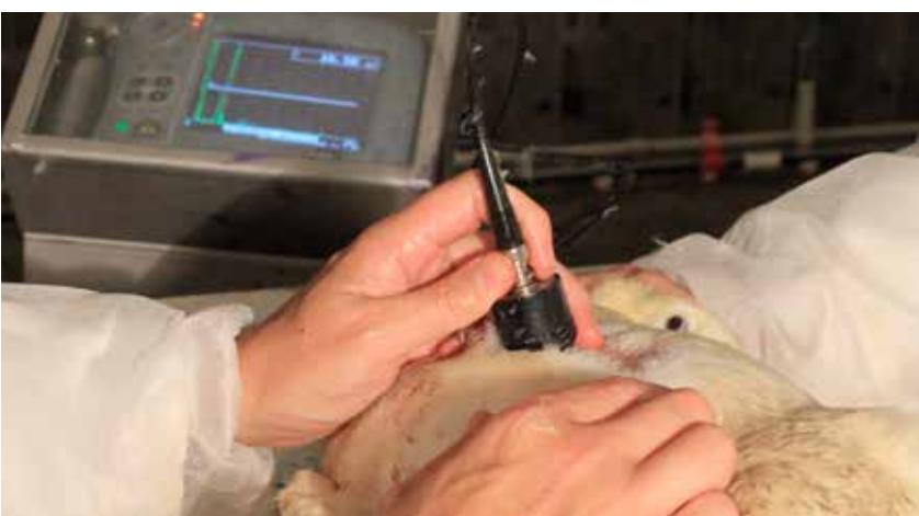
Fig. 2: Breast Thickness is measured using ultrasonic technique
