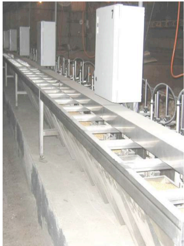
Fig. 1 & 2: Feeding Station to measure individual feed intake in free moving flocks.
