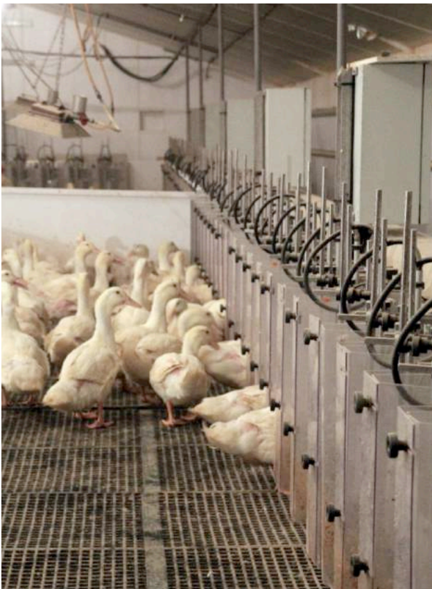
Fig. 1 & 2: Feeding Station to measure individual feed intake in free moving flocks.
